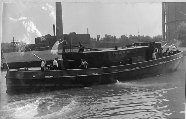
ENGINE - 41 Fireboat "Fred Busse" cruises out into the south branch of the Chicago River from her berth at 23 RD Street Bridge near Throop Street in BRIDGEPORT. The "Busse" was commissioned in 1937, and assigned as Engine 37, built in that year by the Christie-Defoe Shipbuilders, and capable of throwing a barrage of 12,000 GPM from her powerful turrets or "guns" as they are referred to. Built long and low to fit under shallow bridges in the city, (RF) circa 1955
