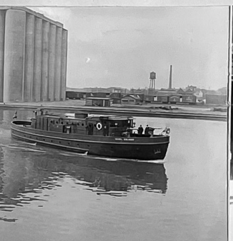
"VICTOR SCHLEAGER" Ewing Ave Bridge at 92nd St 1949 Defoe-Christy 14,000 GPM
