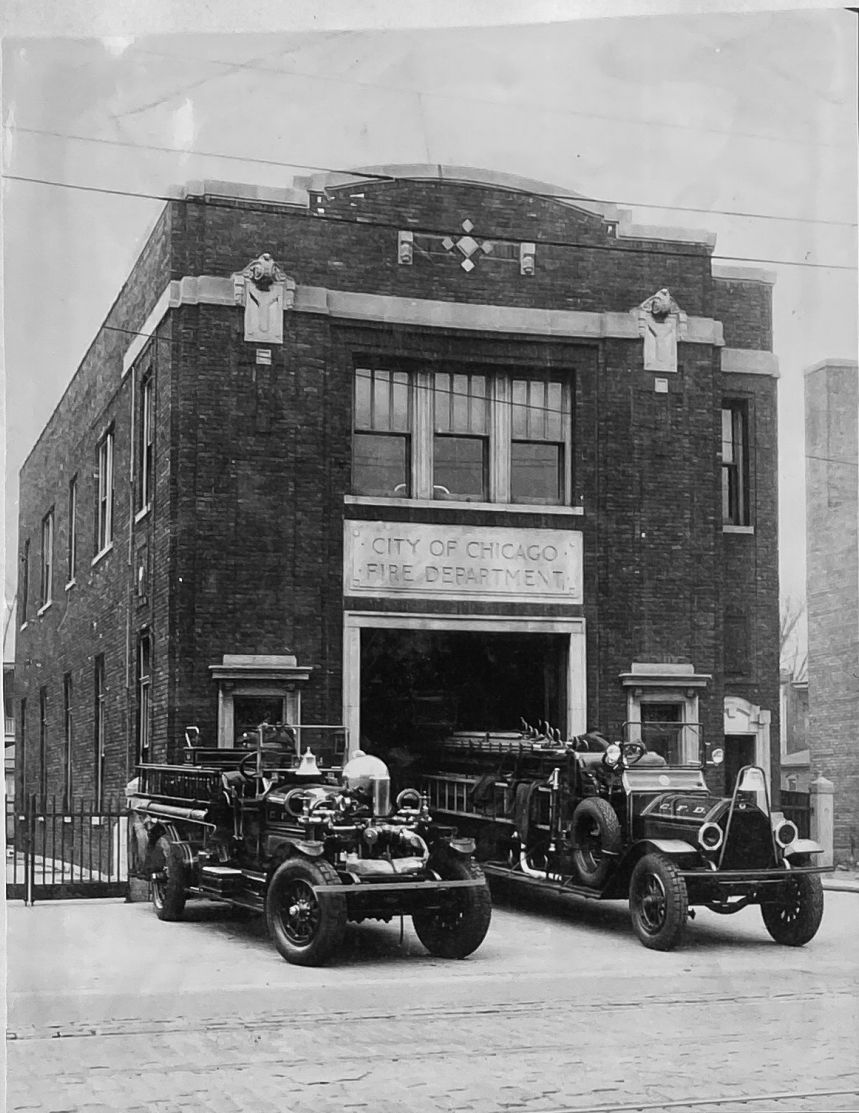
ENG 124 (1922) AHRENS-FOX 750 GPM - TRK 38 (1916) SEAGRAVE EST IN PRESENT HOUSE AT 4426 N. KEORIE AVENUE. NOTE "TALLER" ON LADDER 38, AS IT WAS ONE OF ONLY (TWO) APPARATUS OF ITS KIND BOUGHT BY CFD, FIRST SEAGRAVE OF THIS TYPE ASSIGNED TO TRUCK 11, AND THEN TO TRUCK 20, IN 1920. ORIGINAL TRUCK ABOVE ASSIGNED TO TRUCK 17 UNTIL TRUCK 38 GOT IT IN 1925.
